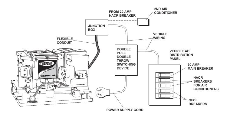
Figure 2.19 — Installation With Isolation Receptacle
